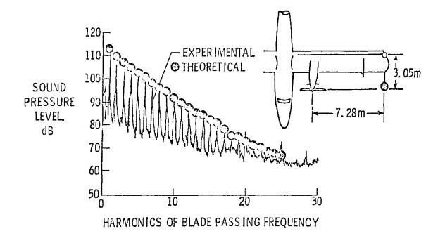
Figure 12.- Comparison of measured and calculated noise levels for a propeller in flight.
